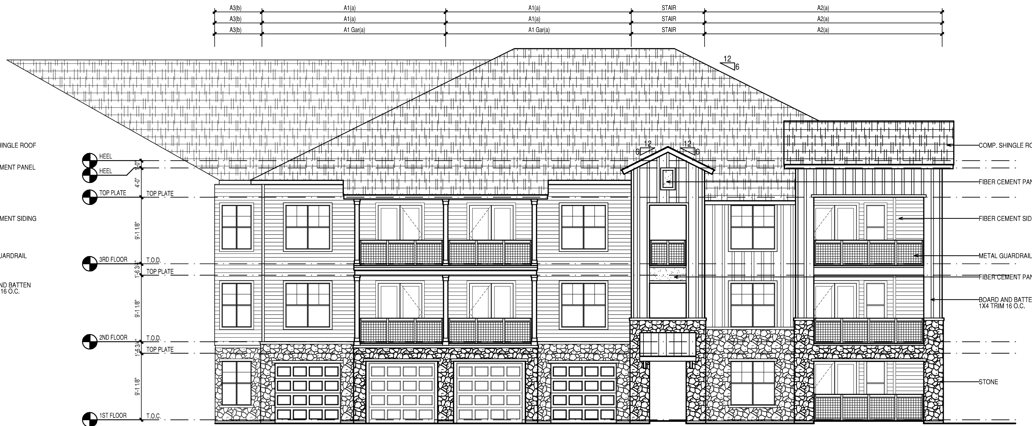
2 BUILDING TYPE 'D' ELEVATION SCALE: 1/8" = 1'-0"
