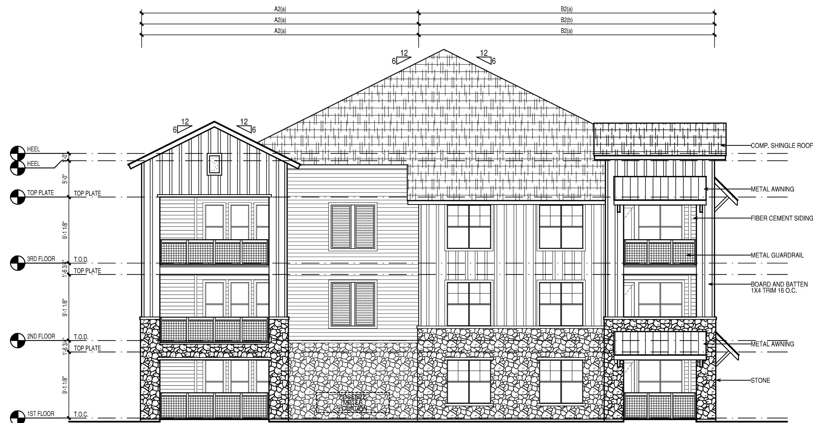
3 BUILDING TYPE 'D' ELEVATION SCALE: 1/8" = 1'-0"
