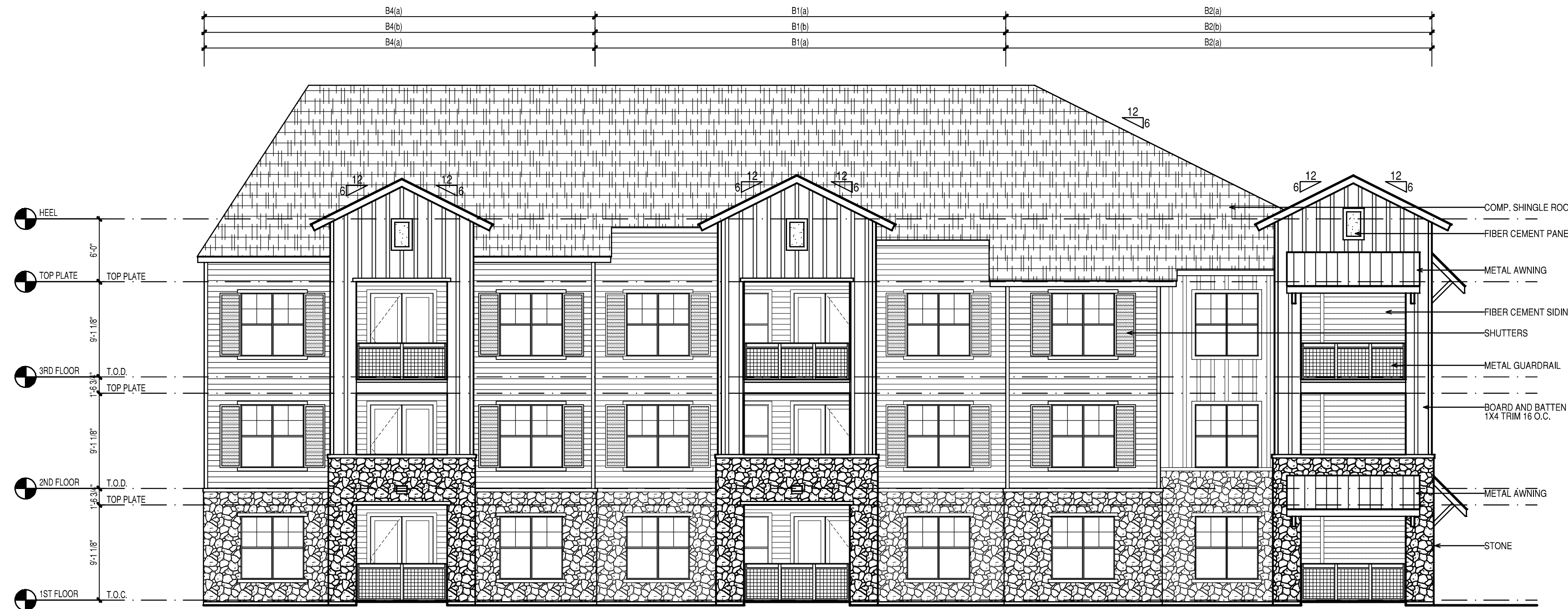
2 BUILDING TYPE 'D' ELEVATION SCALE: 1/8" = 1'-0"
