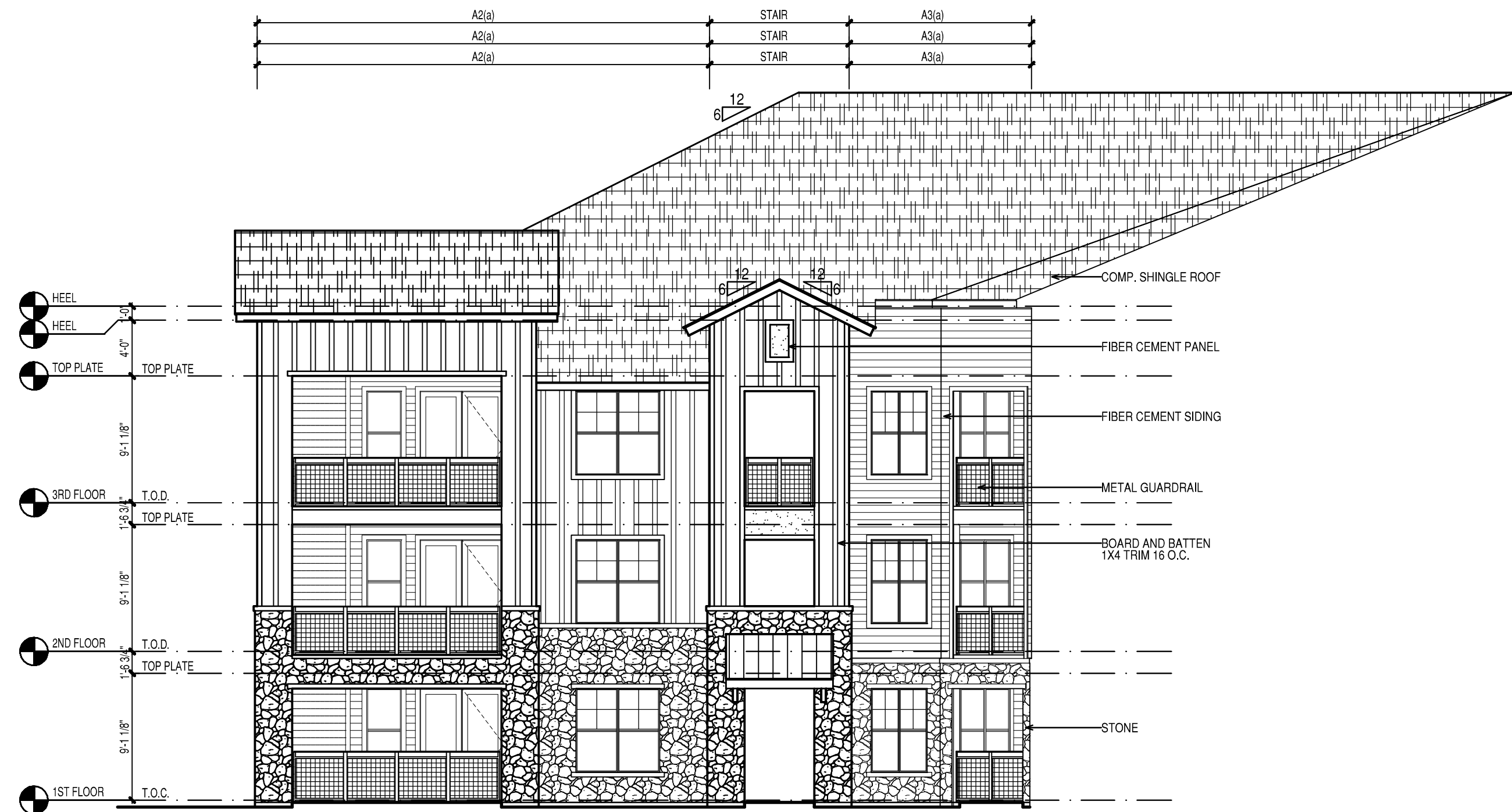
1 BUILDING TYPE 'B' ELEVATION SCALE: 1/8" = 1'-0"
