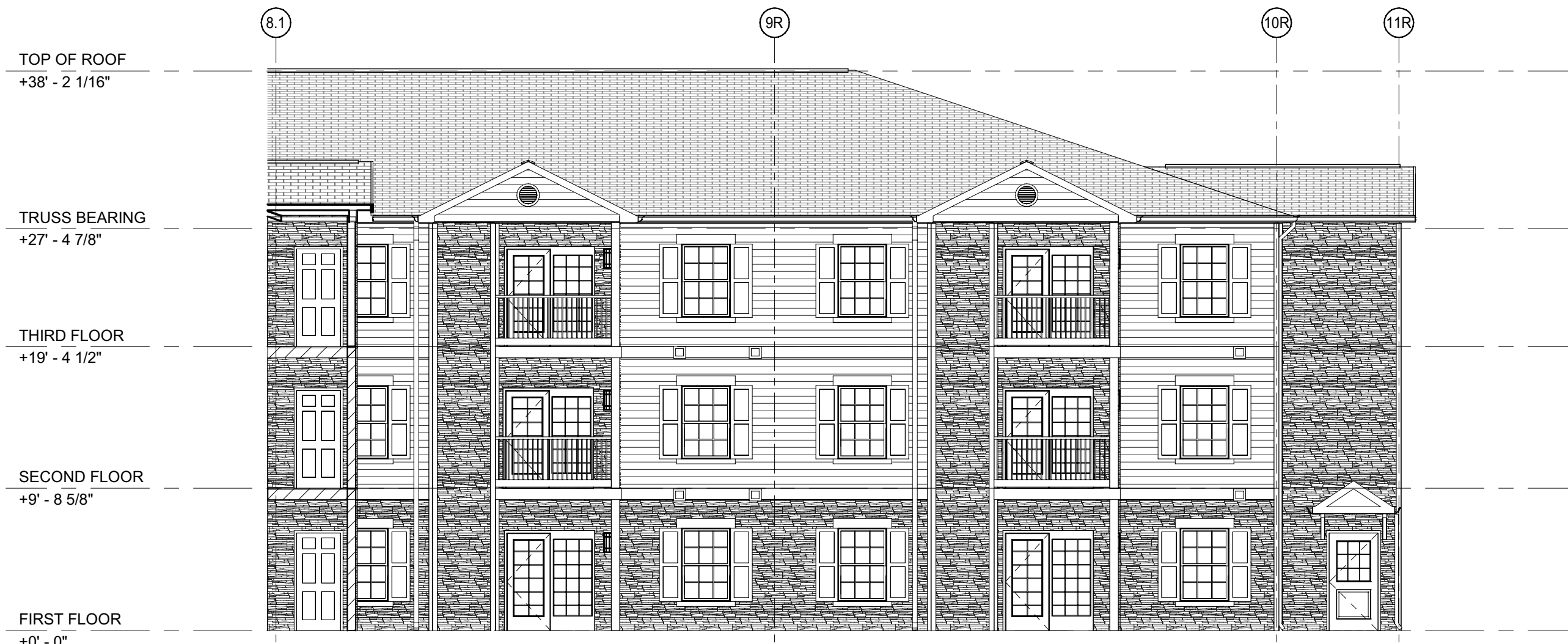
2 Exterior Elevation East Wing - Southwest Face 1/8" = 1'-0"
