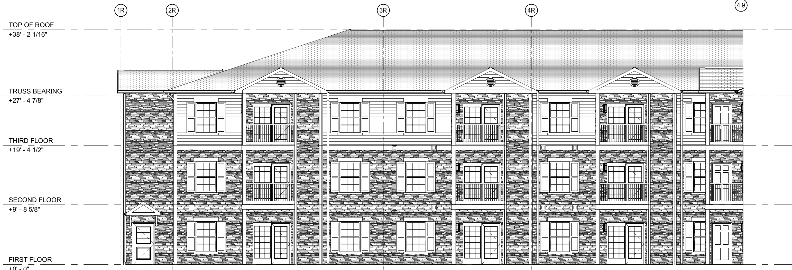
3 Exterior Elevation East Wing - Northwest Face 1/8" = 1'-0"
