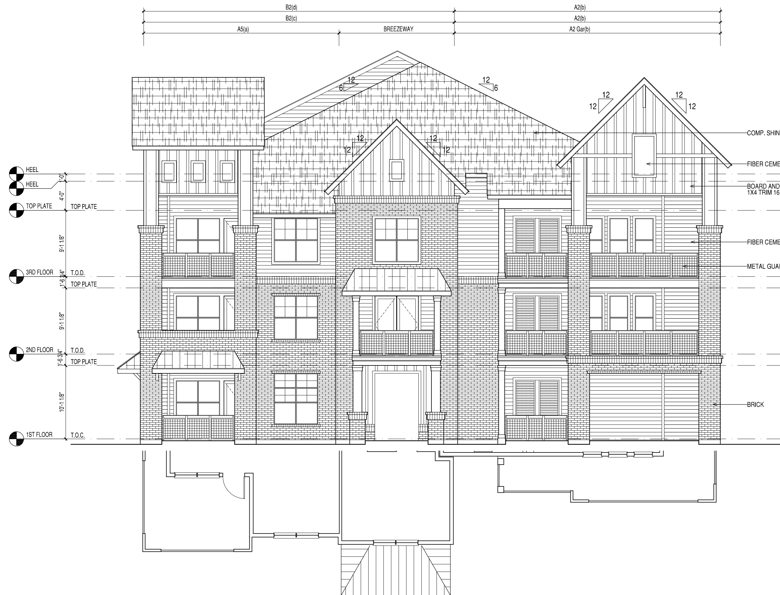
2 BUILDING TYPE 'A' ELEVATION SCALE: 1/8" = 1'-0"
