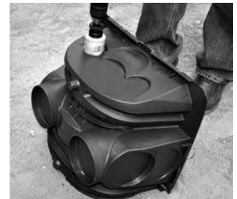
3. Drill pressure pipe location.
