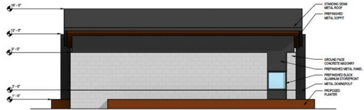
4 NORTH ELEVATION - COMFORT STATION OPTION 1 A201 SCALE: 1/4" = 1'-0"
