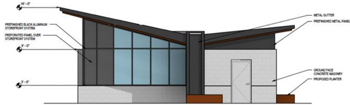
1 EAST ELEVATION - COMFORT STATION OPTION 1 A201 SCALE: 1/4" = 1'-0"
