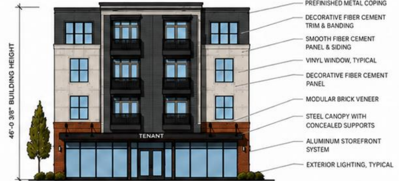
4 SIDE ELEVATION (RIGHT - STOREFRONT END)
