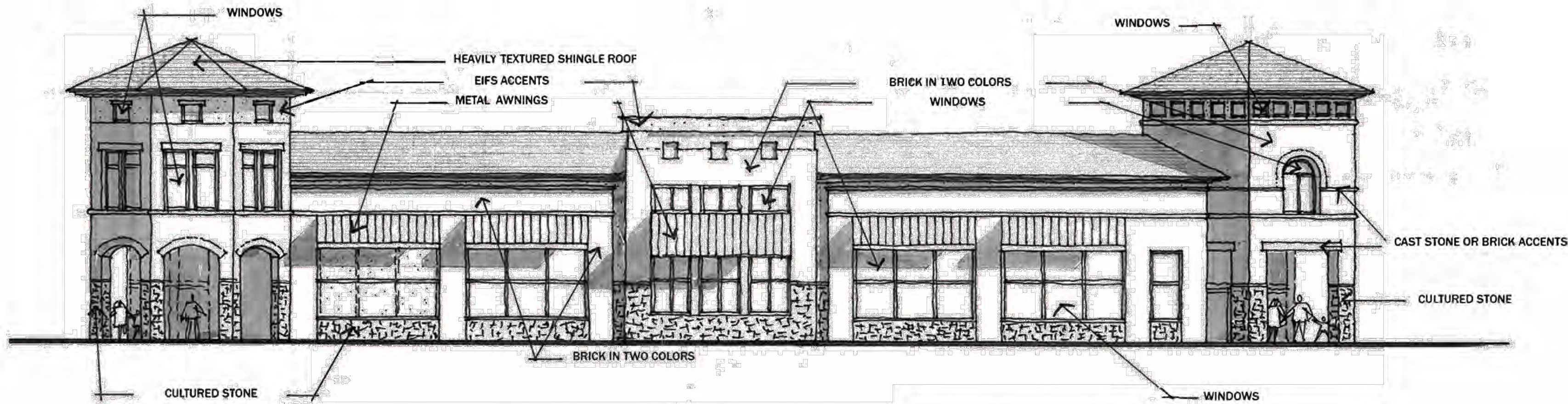
01 BUILDING H - (PHARMACY) EASTFIELD RD ELEVATION 3/32" = 1'-0"
